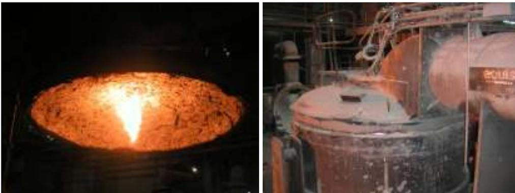
Figure 13. Ladle drying and preheating with flameless oxyfuel at Acerinox, Spain.
