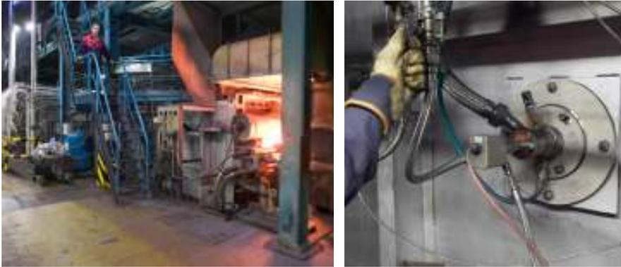
Figure 9. Flameless oxyfuel burner installation at Outokumpu Nyby.
