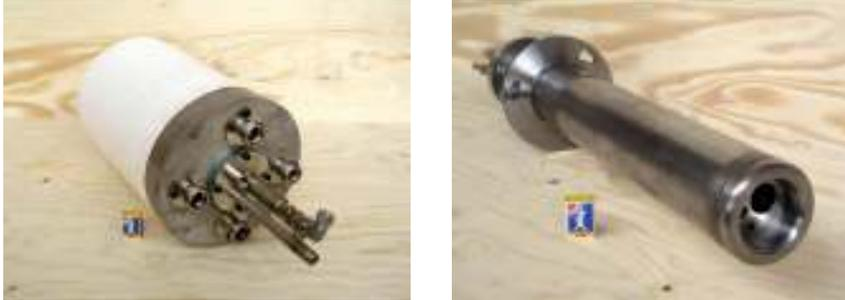
Figure 6. The photo to the left shows a 3 MW, self-cooled ceramic flameless oxyfuel burner. To the right is a compact 5 MW water-cooled flameless oxyfuel burner displayed. Both are equipped with an integrated UV cell and a pilot burner. The reference object is a matchbox.
