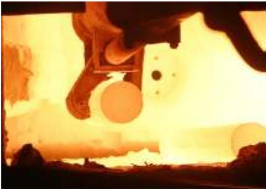
Figure 11. A look through the door into the flameless oxyfuel fired rotary hearth furnace at ArcelorMittal, Shelby.
