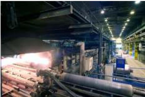
Figure 10. Flameless oxyfuel burner installation at Outokumpu Avesta Works.
