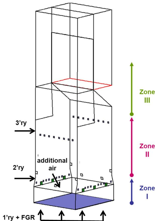
Figure 1. Air staging in BFB and the three combustion zones
