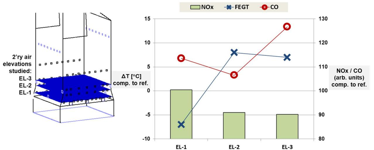
Figure 5. CFD results: effect of 2<sup>ry</sup> air elevation with additional air feed
