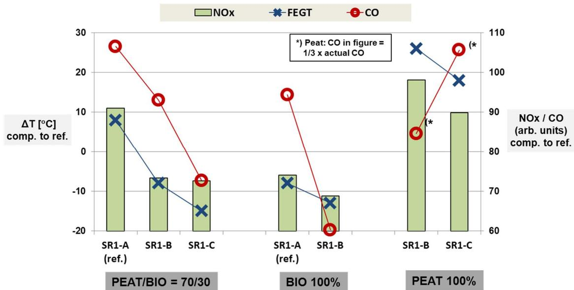
**Figure 6. CFD results: effect of Zone I stoichiometry with additional air feed. SR1-A < SR1-B < SR1-C**
