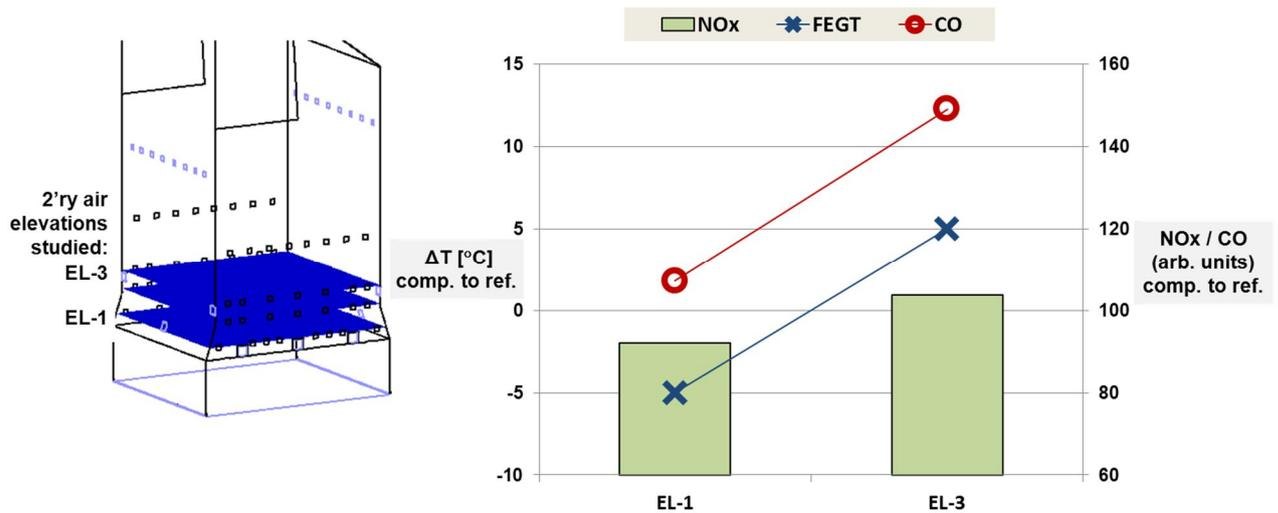
Figure 4. CFD results: effect of 2<sup>ry</sup> air elevation, no additional air feed
