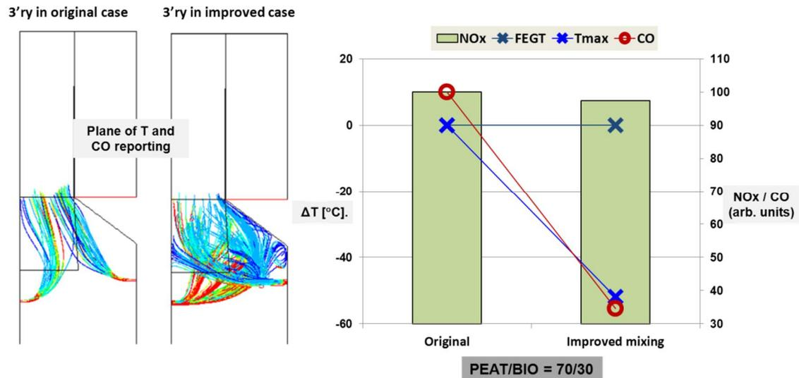
Figure 7. CFD results: mixing study
