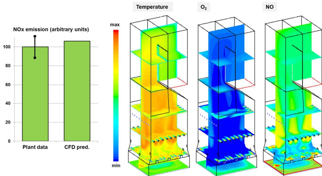
**Figure 3. CFD results from the reference case (validation)**
