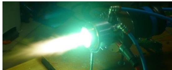
Figure 3. Plasma torch PW 15 with a nominal power of 15 kW.
