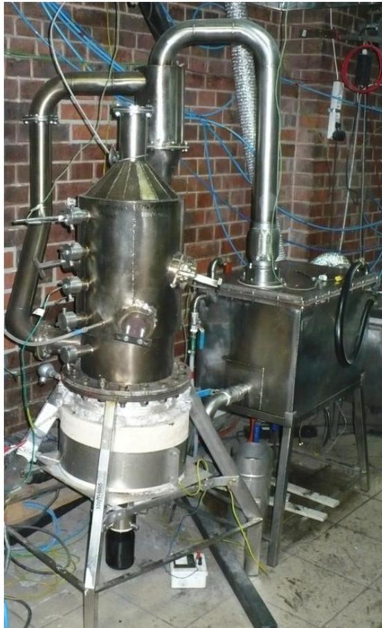
**Figure 4. View of the fundamental elements of the plant used in a plasma gasification of wastes.**
