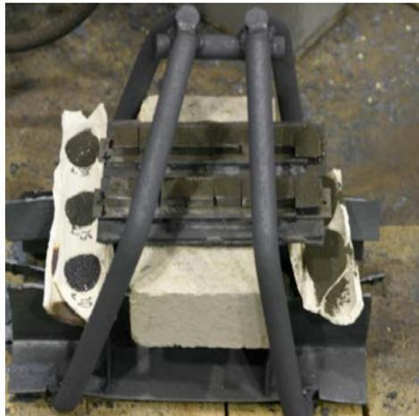
Figure 2. Ash on steel specimens and as an ash plus steel scale powder on alumina holders before entering the furnace
