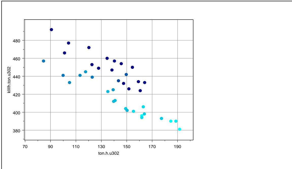
**Figure 2.** The fuel consumption is shown as a function of the oxygen use. Dark blue=no oxygen use, light blue= oxygen up to 4000 m<sup>3</sup>/h.
