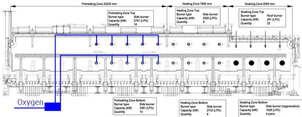
Figure 4. Walking beam furnace at Outokumpu. Twenty HLL lances are installed in the upper and lower preheating zones.
