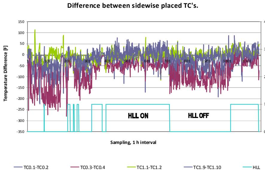
**Figure 3. The impact of the HLL operation on the zone's deviation in temperature distribution.**
