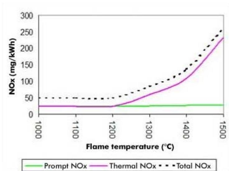
**Figure 1. NOx formation in relation to the flame temperature (Article in Tecno Impianti).**
