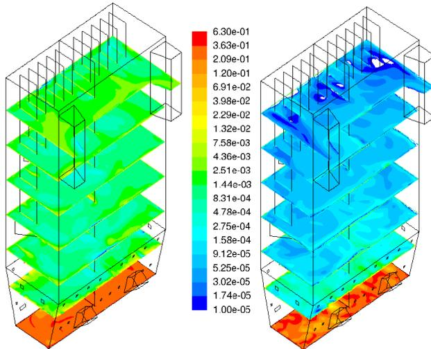
**Figure 4. Solids volume fraction contour at 120 MWe (left) and 80 MWe loads.**
