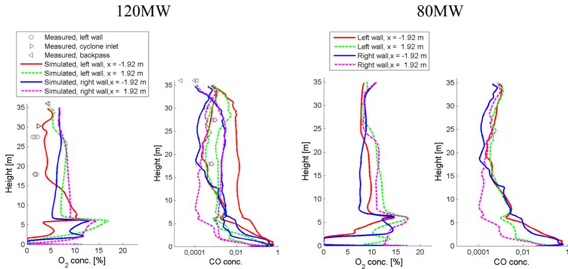
**Figure 5. Comparison of simulated vertical O<sub>2</sub> and CO concentration profiles to measured values at 120 MWe load and the simulated profiles at 80 MWe load.**
