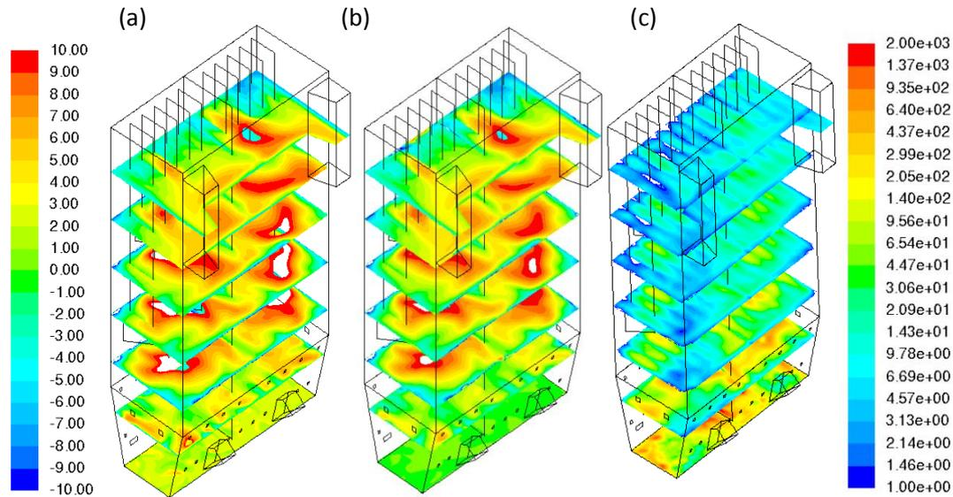
**Figure 3.** Contours of simulated gas (a) and solids (b) vertical velocities [m/s] and (c) net heat of reactions [W/cell] at 80 MWe load.
