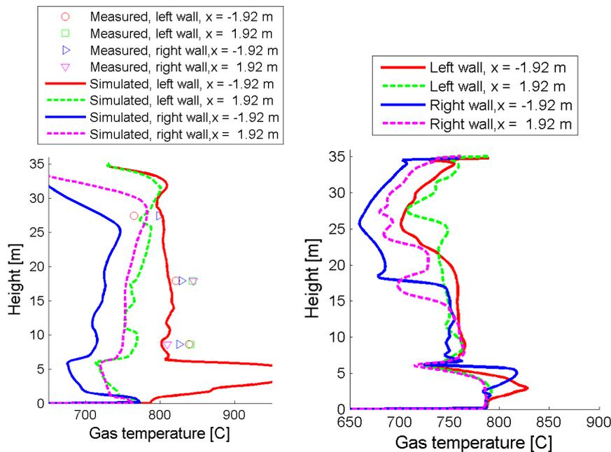
**Figure 6. Comparison of simulated vertical gas temperature profiles to measured values at 120 MWe load (left) and corresponding simulated profiles at 80 MWe load (right) in the vicinity of the side walls.**
