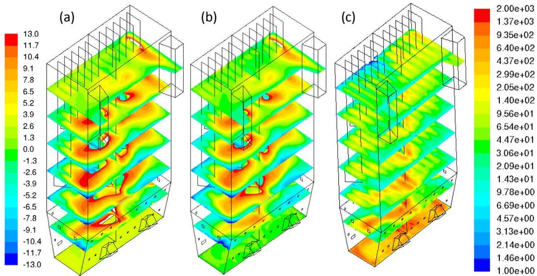
**Figure 2.** Contours of simulated gas (a) and solids (b) vertical velocities [m/s] and (c) net heat of reaction [W/cell] at 120 MWe load.
